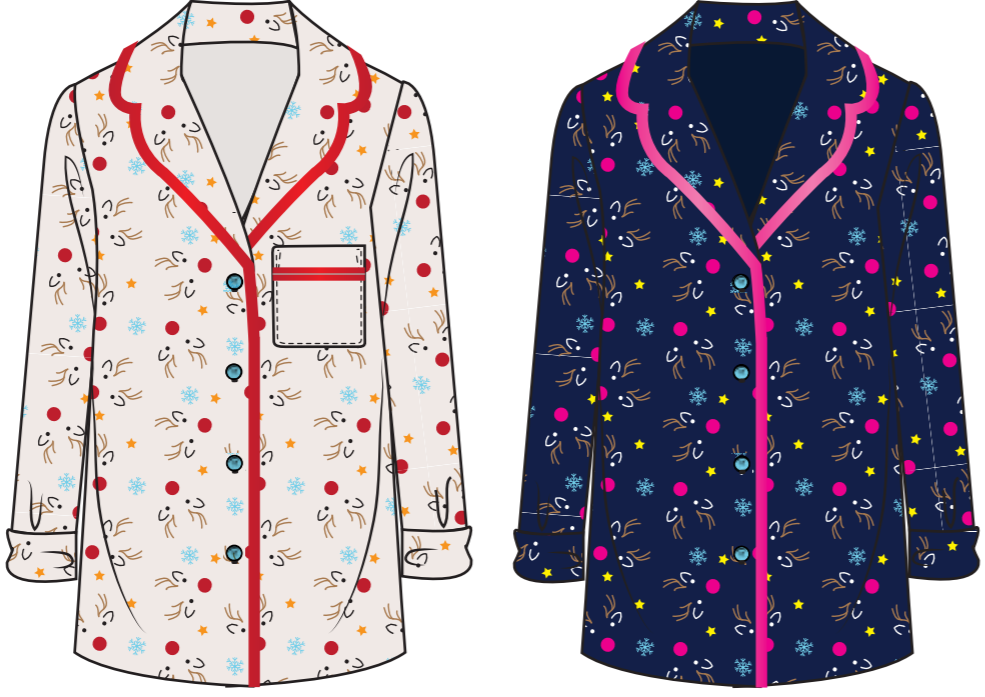
100% COTTON AOP SHIRT WITH SATIN CONTRAST PIPING. PLASTIC CONTRAST BUTTONS. PLAIN PATCH POCKET.
